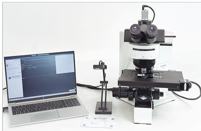
Example autoWSI configuration: Microscope with motorized XYZ stage and digital camera, connected to a PC running autoWSI. Optional Macro Camera for label and slide imaging.
